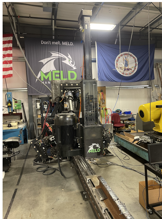
Fig. 1 The Hexapod and Rail Mover system
