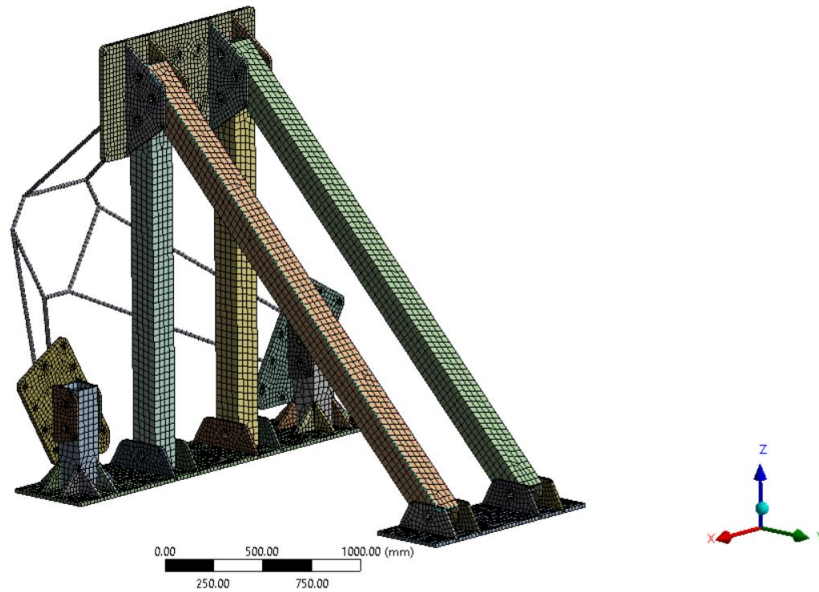
Fig. 18 Mesh with 8 mm*-node Quadrilateral elements
